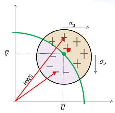
Points are couple of U and V measured over 10 minutes, red arrow are example of vector with the HWS scalar value and green line is a constant HWS value curve
