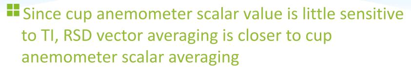
$$HWS_{RSD_{vector}} = \sqrt{\overline{u_{center}}^2 + \overline{v_{center}}^2}$$
